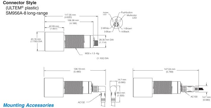
AC130, Straight, M12 micro, 4-conductor, connector/cable assembly, 5 m (16), for 30 mm, barrel-style sensors
