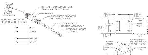
AC132, Right-angle, M12 micro, 4-conductor, connector/cable assembly, 5 m (16'), for 30 mm, barrel-style sensors
