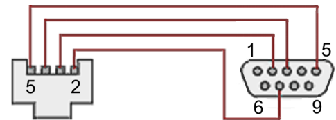
RJ11-to-DB9 RS232 cable with rear view of DB9 connector to PC
