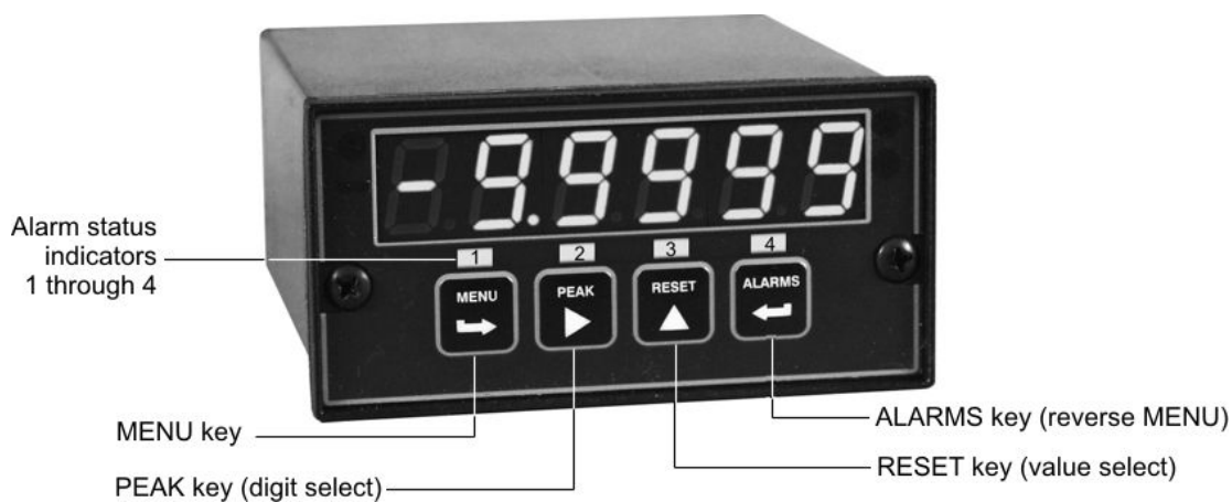
Meter Front Panel
